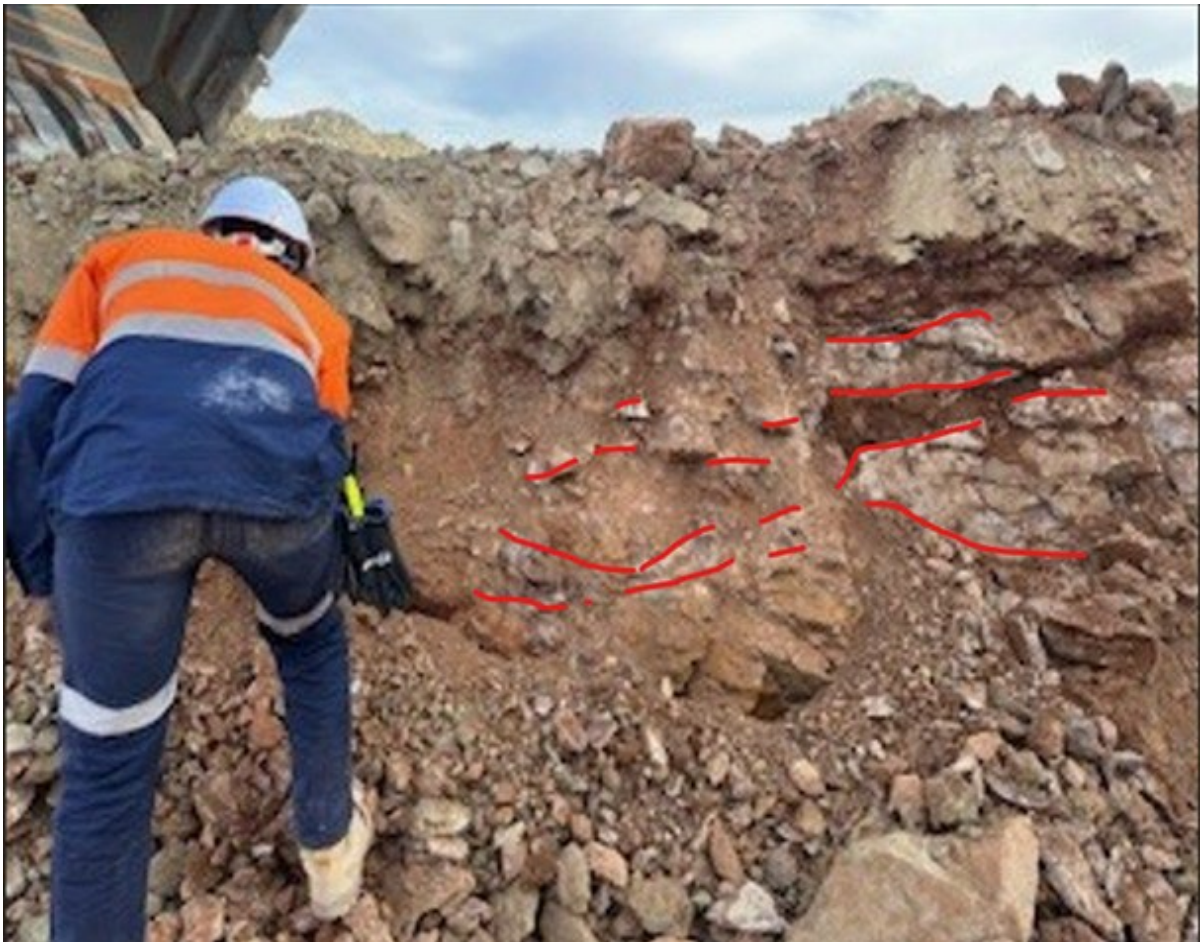
Plates 6 & 7 ROM Pad layout (top) and ore mapping showing pinch and swell structures (bottom)
