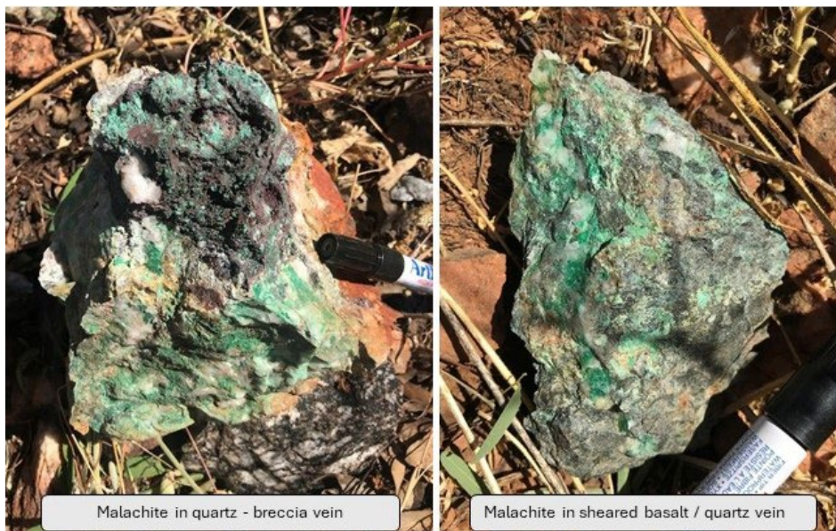
Figure 4. (Left and right) Example of the copper mineralisation identified in rock samples collected for assay
