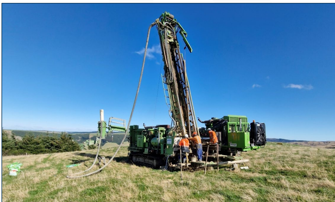
Figure 10: Photo of RC drilling operation on Waipori Station (EP60807 - Lammerlaw)
