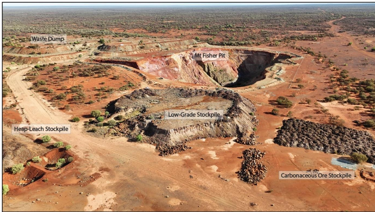
Figure 1- Image looking north-west showing historical pit, waste dumps and stockpiles.
