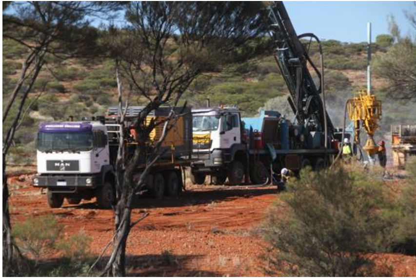
Picture 1: RC drilling team drilling at Smokebush gold project at the Lightning & Monza parallel structures.
