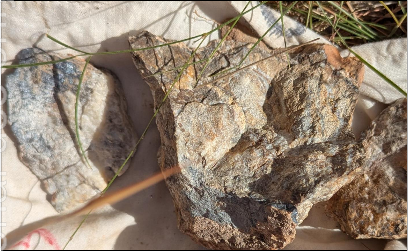
Figure 3. Rock chip sample IRX00088 from Bouncer South, returning 6.44 g/t Au and 6.53% Sb. Sample comprises quartz-sulphide veining with abundant stibnite, consistent with high-grade antimony mineralisation.
