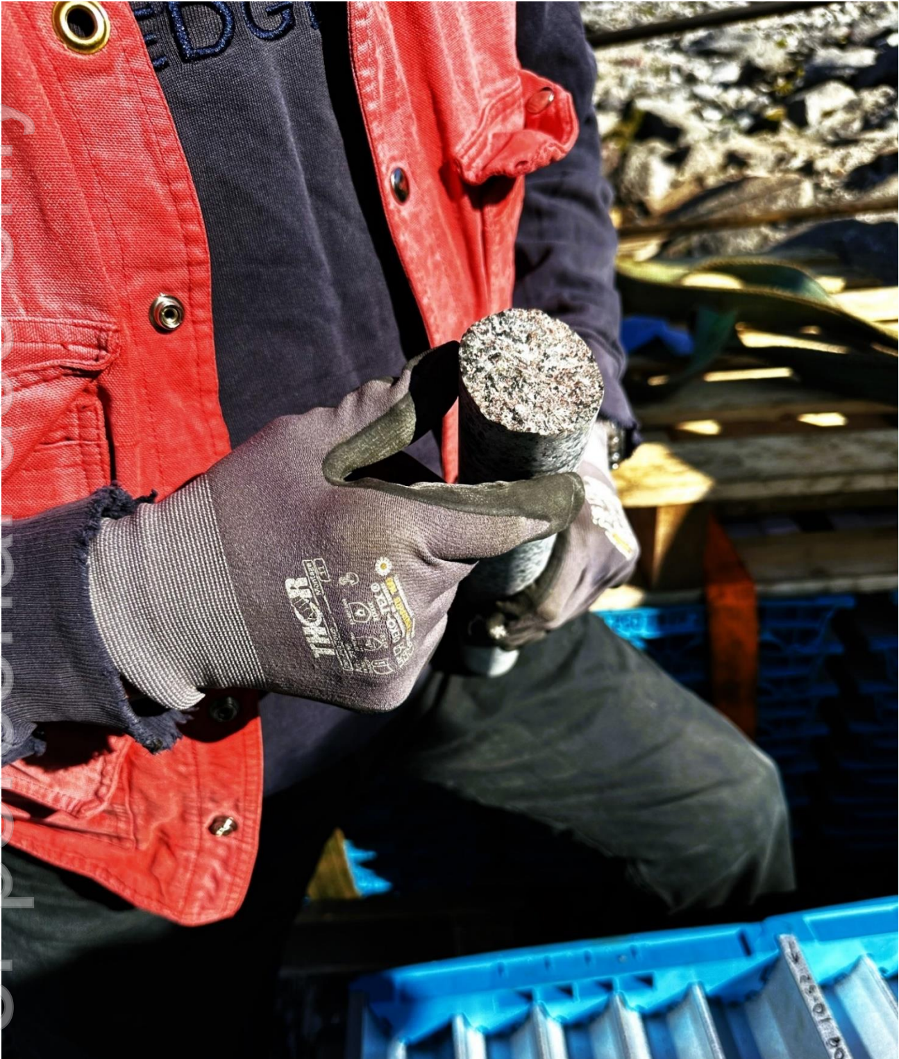
Figure 2. Drill core K25-01 in kakortokite host from surface to current depth of 61m, composing continuous medium grained red - mauve eudialyte mineralisation
