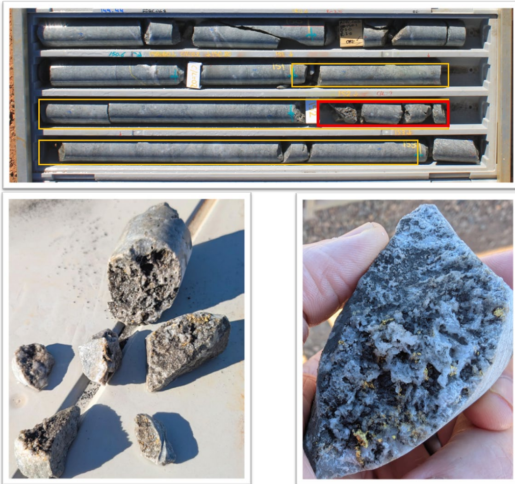
Figure 3: [TOP] shows the core from RDRC068, 149.44m to 153.13m, the yellow box highlights the interval 2m @116.3g/t from 151m to 153 m. The red box highlights the interval 0.2m @ 1,148 g/t Au from 152m-152.2m. [BOTTOM_LEFT] shows some core pieces from 152m-152.2m. [BOTTOM_RIGHT] shows a close-up of one of the pieces of core from the Bottom-Left figure with visible gold.
