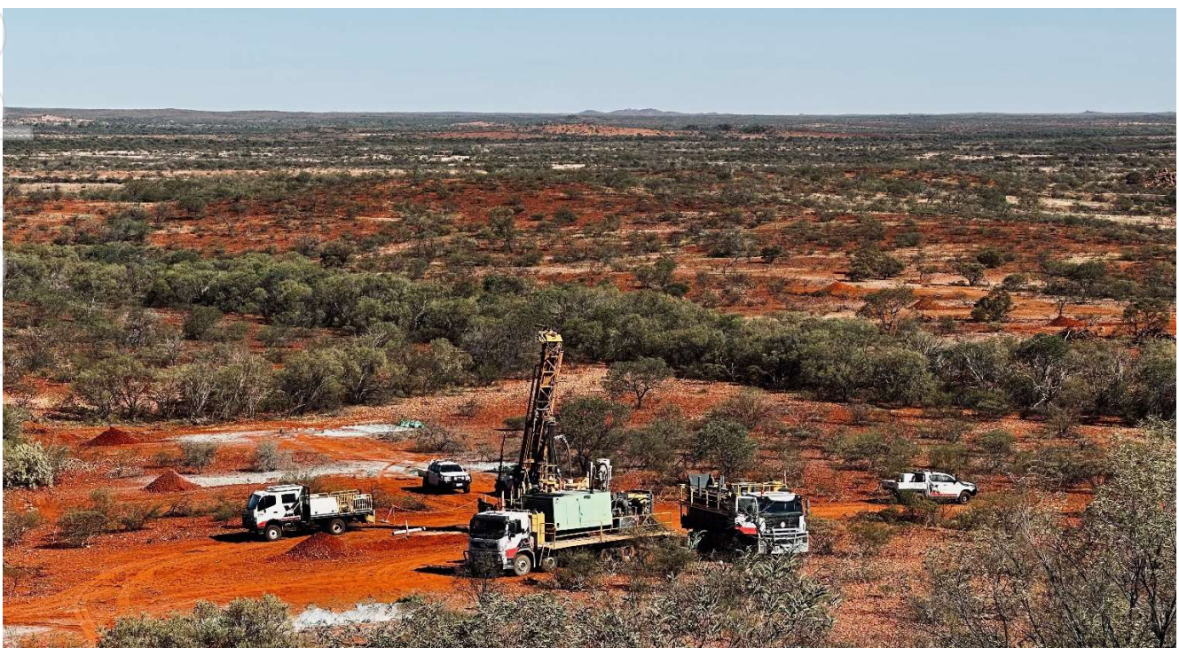
Figure 1: RC Rig Drilling at Steve’s Reward
