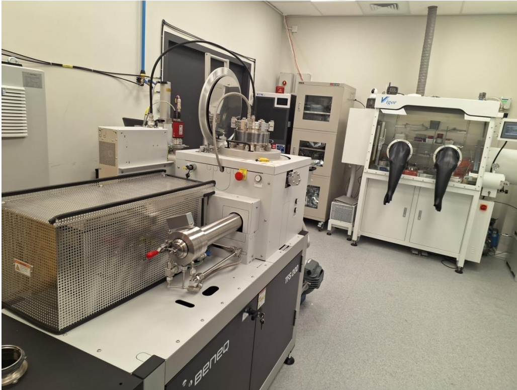
Figure 2: 2DG Process Room featuring Beneq TFS 200 ALD system and associated glove box (Yakum Industrial Park, Israel)
