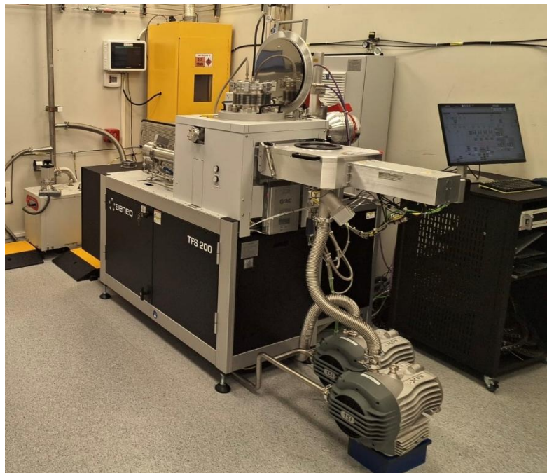
Figure 1: Successfully commissioned Atomic Layer Deposition system at 2DG lab at Yakum Industrial Park, Israel
