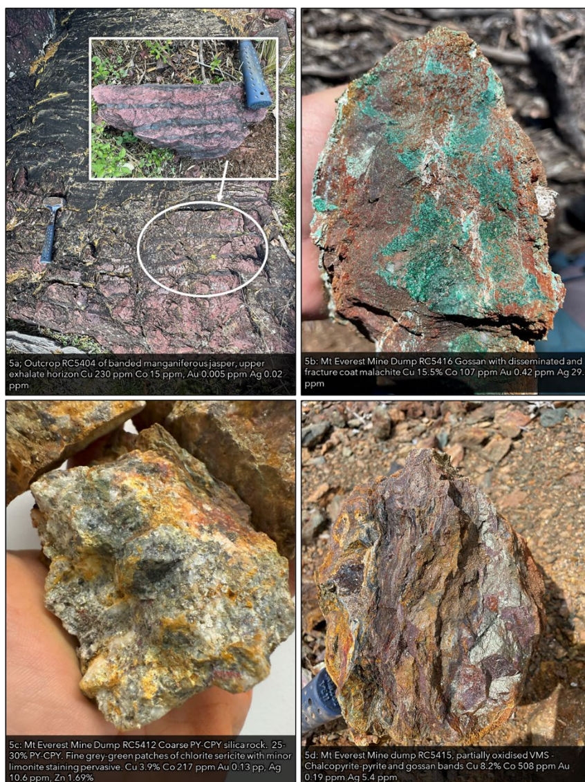
Figure 5. Mt Everest Mine selected Outcrop and Dump Samples (see Appendix 1, Table 1 for details)
