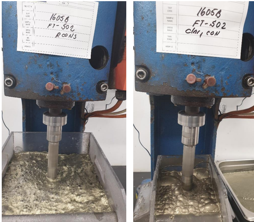
Figure 4: Copper concentrate from Kabikupa fresh composite – chalcopyrite is the major copper mineral
