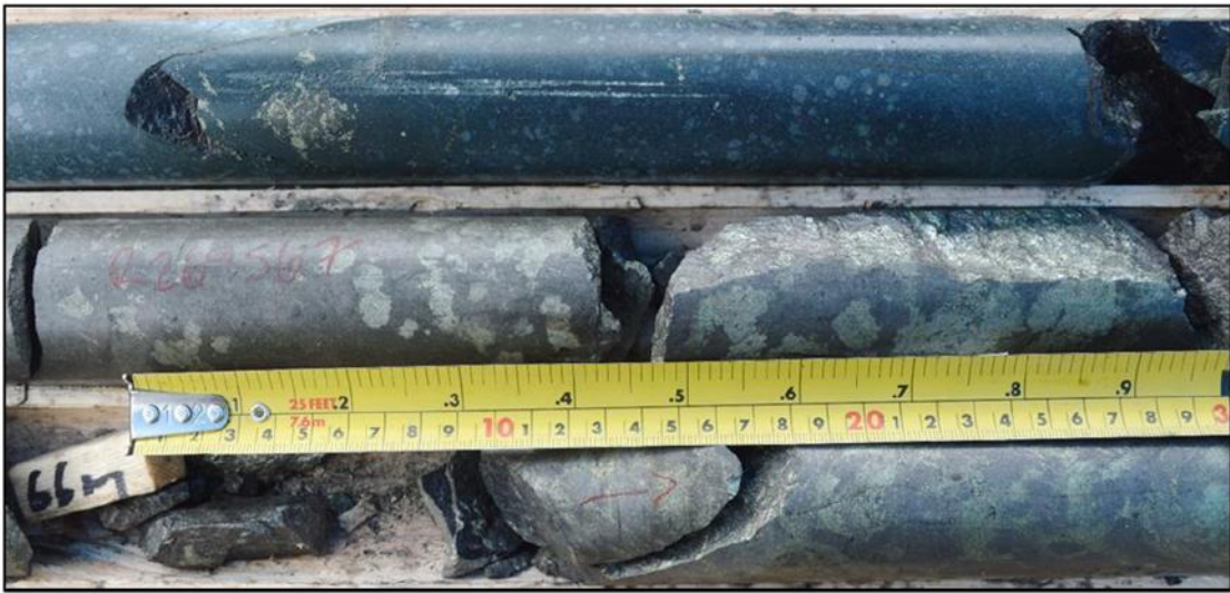
Figure 3: Massive pyrrhotite with coarse pyrite and disseminated chalcopyrite. Alotta occurrence drill hole 20-ZA-01, composite 63.70-67.00m. Refer Table 1 for assay results.
