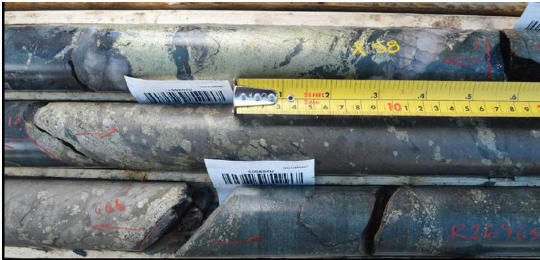
Figure 4: Massive chalcopyrite and massive pyrrhotite with coarse pyrite. Alotta occurrences drill hole 20-ZA-05, composite 57.00-62.30m. Refer Table 1 for assay results.
