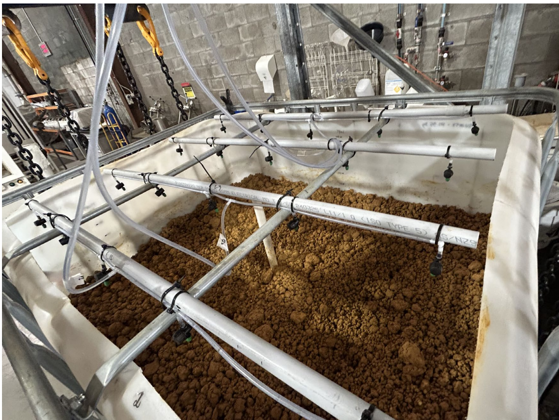
Figure 2: Bulk Leach with dripper system applying lixiviant for leaching
