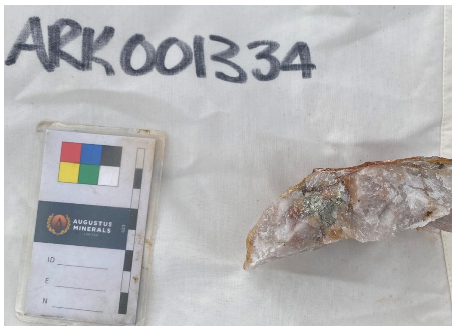
Figure 6 Teutonic East sample which assayed 62.2g/t Au comprised of crystalline quartz with fresh pyrite (brassy-grey metallic mineral in photo).
