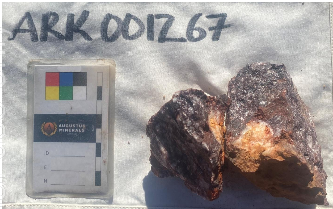
Figure 8 Dodd's sample which assayed 8.17/t Au comprised of brecciated ferruginous quartz.
