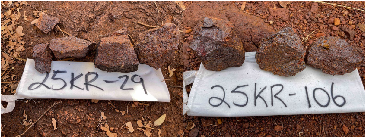
Image 1 and 2: Typical CID material, sample 25KR-29 assayed 60.59% Fe and sample 25KR-106 assayed 60.68% Fe (Appendix 1).
