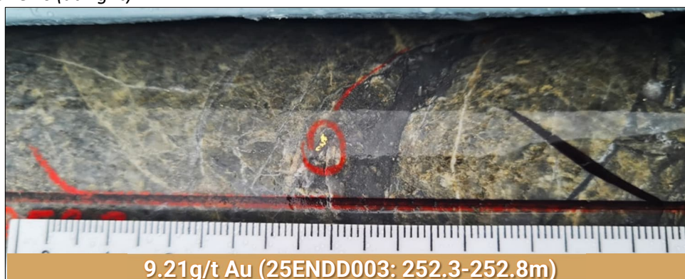
Photo 3. Sample photo of 25ENDD003 from 252.3m – 252.8m @ 9.21g/t Au with visible gold circled in red associated with very fine-grained pyrite-arsenopyrite-arsenian pyrite vein (dark colour). 3
