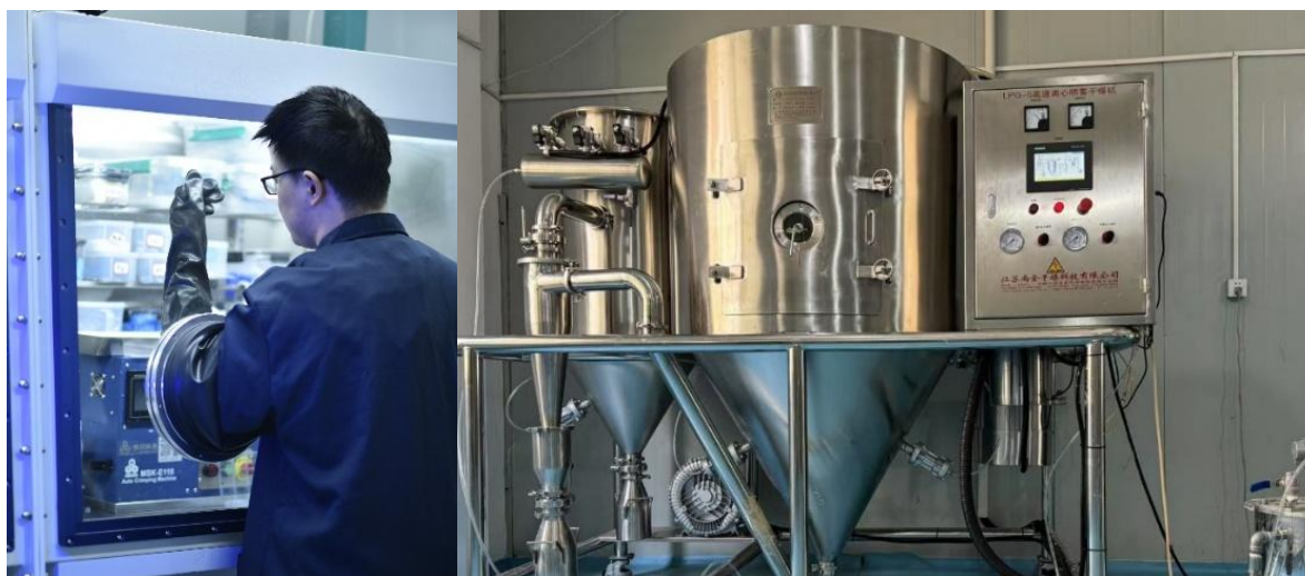
Images 2 and 3: Lab cell test work and CAM production equipment (Spray Dryer)
