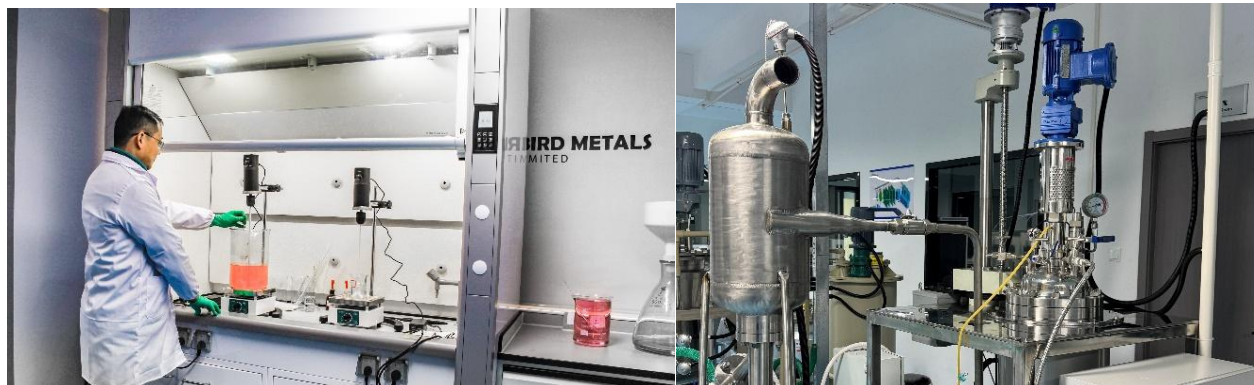
Images 4 and 5: Manganese sulphate process and crystalliser reactor
