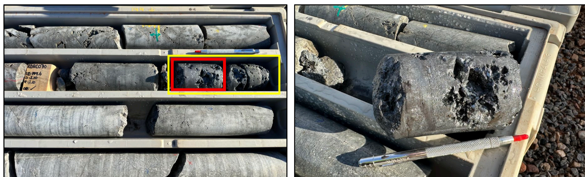
Figure 2: [Left] shows selected core from the RDRC070 coretray: 148.26-151.75m, which is part of the significant interval: 22.8m @ 1.95 g/t Au and 0.68% Sb from 140m (RDRC070), including 4m @ 8.69 g/t and 3.29% Sb from 146m. The yellow box highlights massive stibnite intersected at 148.8m. The red box is massive stibnite, shown in the photo on the right. [RIGHT] shows a close-up of one of the pieces of massive stibnite highlighted by the red box in the photo on the left.
