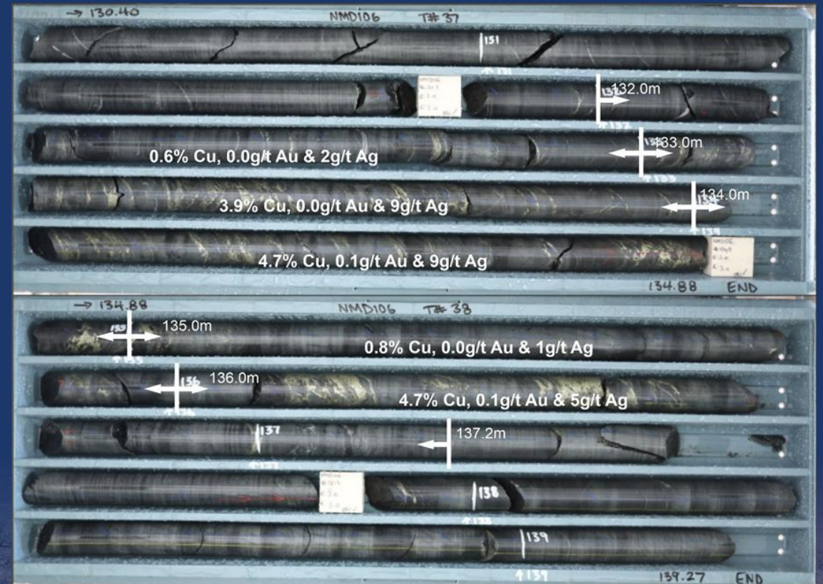
Photo: Nymagee drill core from drillhole NMD106, between 130.4m and 139.3m showing significant intersections
