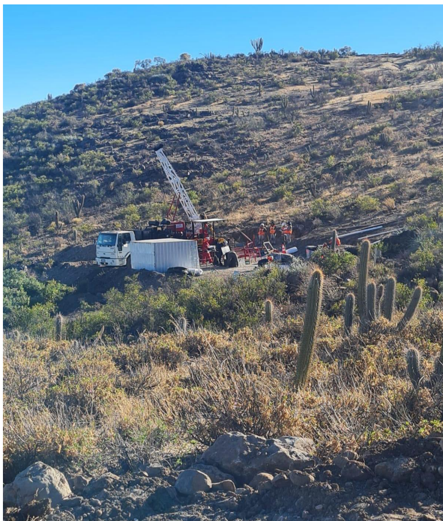
Figure 4: Drill rig on platform 2025FL02 drilling maiden diamond hole CMLFD001.
