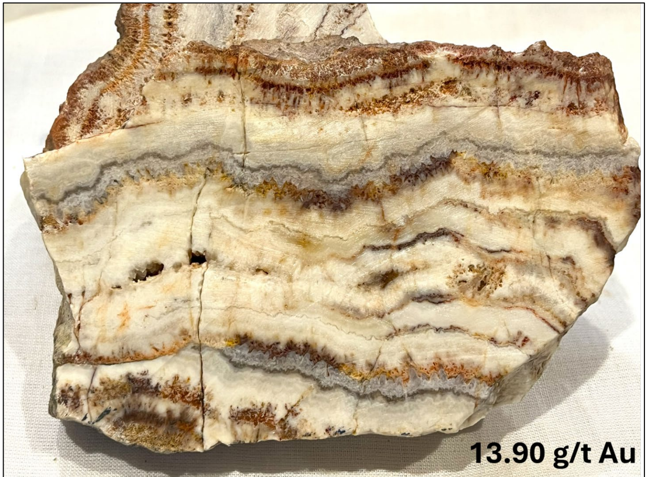
Figure 4: Crustiform - colloform banded quartz-adularia vein. Rock chip (sample FC25_013) that assayed 13.90g/t Au, from Francis Creek.
