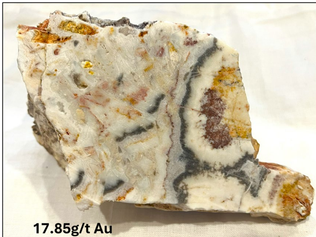
Figure 1: Brecciated crustiform-colloform silica-sulphide banded quartz vein. Rock chip (sample FC25_005) that assayed 17.85g/t Au, from Francis Creek.
