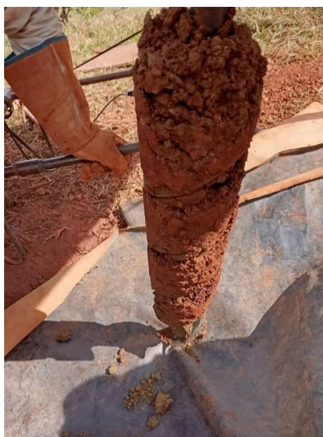
Figure 5: Kamafugite red saprolite with titanium and REE mineralisation in CODA Central - CDC-AD-0005
