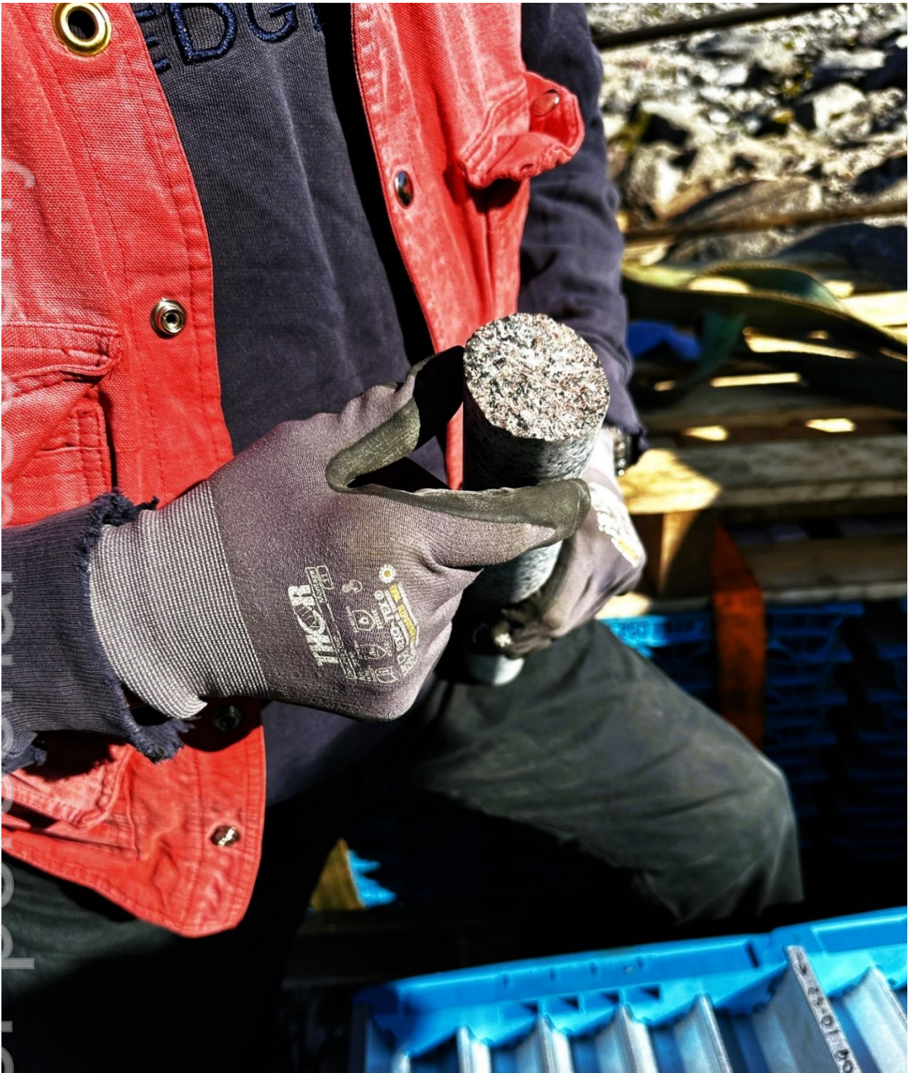
Figure 2. Drill Core drill hole DDH K25-01 is metasomatized kakortokite host rock from surface and the core photographed from the current depth of 61m. The kakortokite is composed of banded fine to medium grained red - mauve Eudialyte ~ 25%, grey to white Sodalite and Nepheline Feldspars ~ 40% and shards of black Arfvedsonite ~ 35%.
