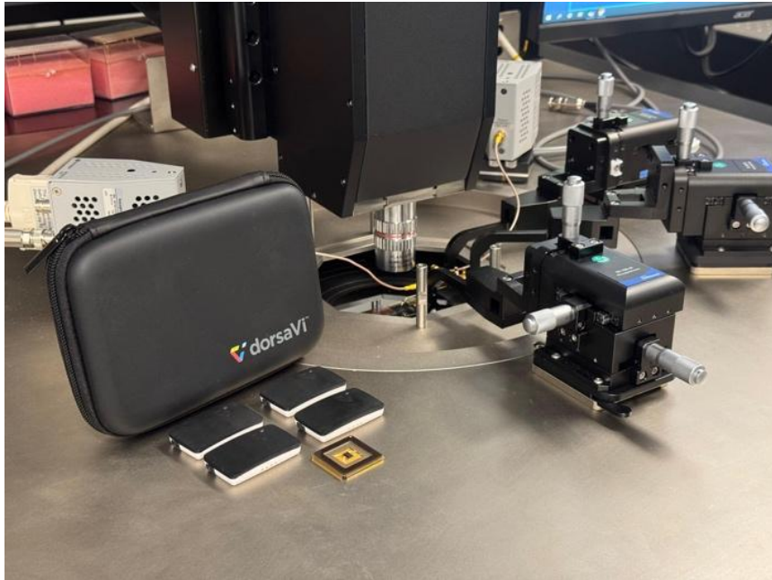
Figure 5: DVL sensor undergoing wafer-level testing
