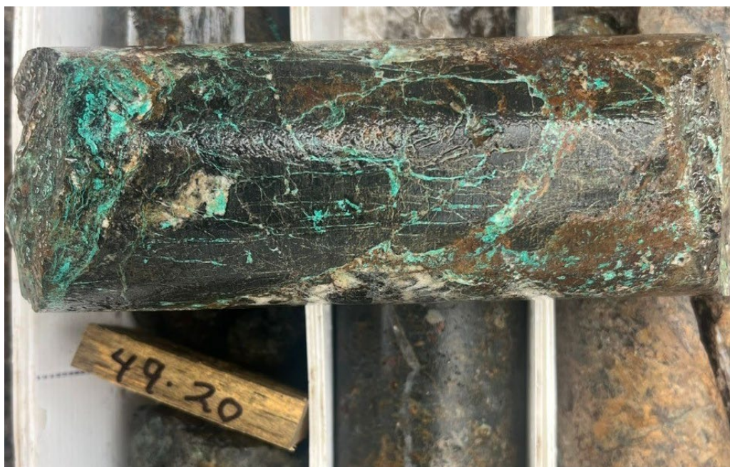
Figure 1: CAP-002-2025 drill core at 49.20 metres displaying tourmaline/specularite breccia with malachite (copper oxide) mineralisation hosted in diorite intrusive. Visually estimated grade 0.5% Cu. Laboratory assays are due in July / August 2025.
