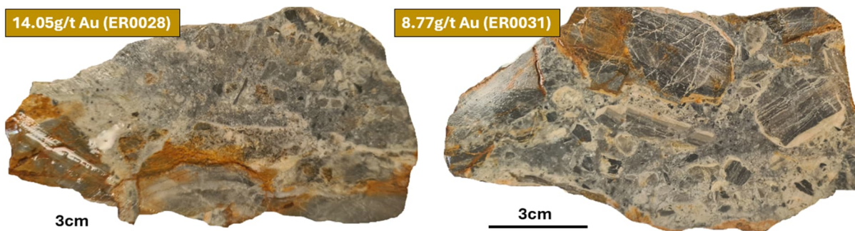
Photo 3 (left). 14.05g/t Au rock chip sample from mullock pile at Postman's Gully Prospect consisting of pervasive quartz-pyrite-sericite altered siltstone breccia with a rock flour matrix containing sulphides, cross cut by hairline quartz veins.
