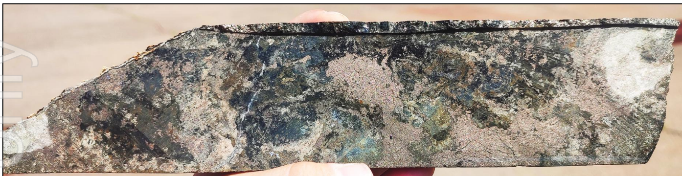
Figure 6. Core photograph from 394.6m in ZRSD25190 showing strong pyrrhotite alteration – 5.0g/t Au.
