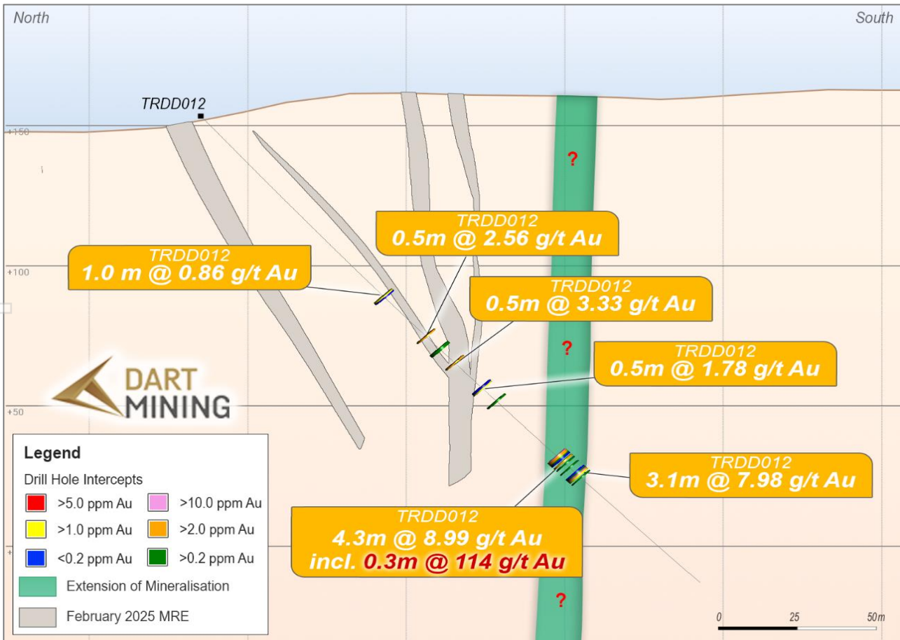
Figure 4: TRDD012 oblique cross section showing projected extension zone of mineralisation in green and assays > 0.1 g/t Au.
