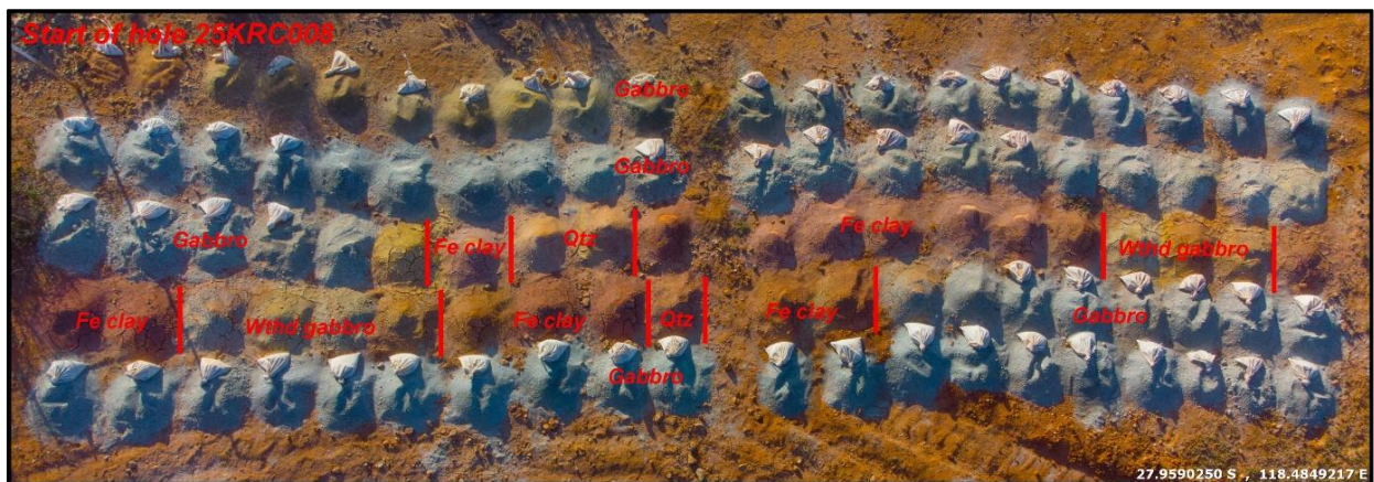
Figure 4: Drillhole 25KRC008 sample piles showing heavily weathered ferruginous material downhole
