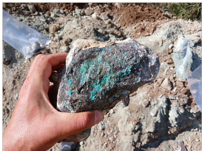
Photo 2: Copper oxides within ferruginous-calcite – DET003 61-62m
