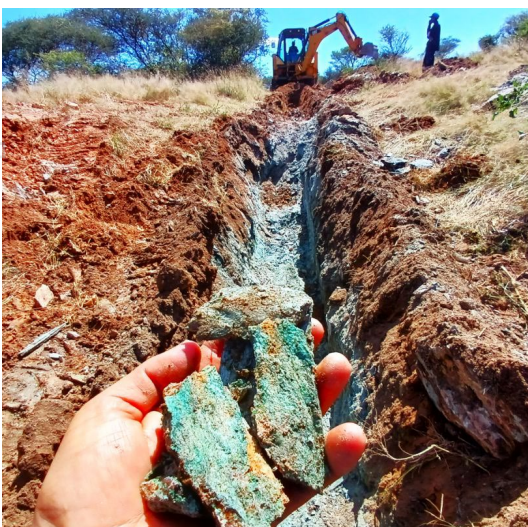
Photo 1: Copper oxide mineralisation in schist – DET003 2-5m
