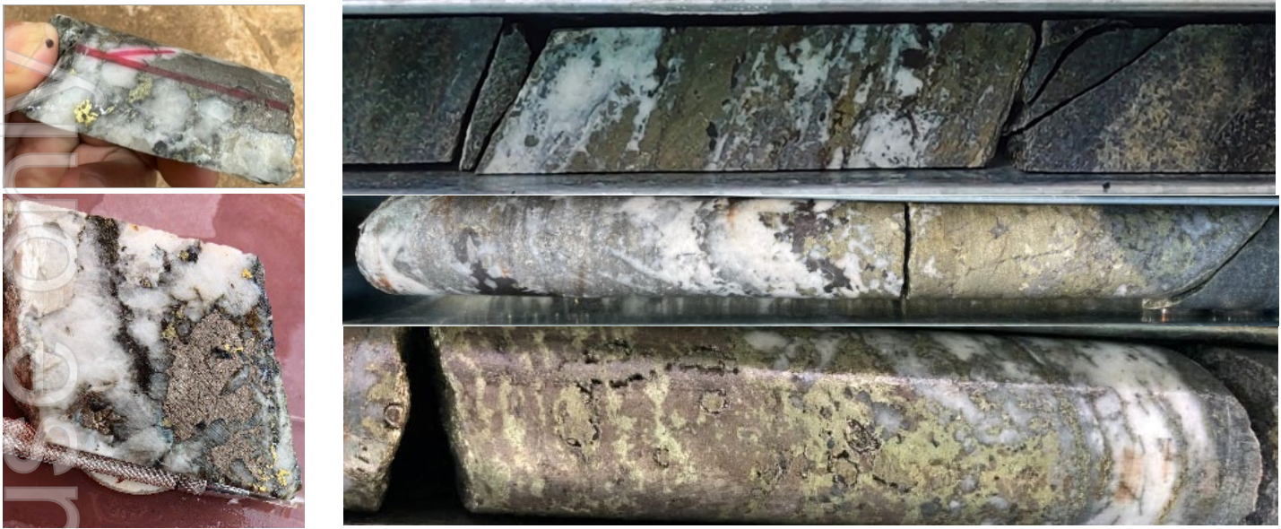
Figure 6 | Mineralised veins in Memot diamond core. Quartz veining with Pyrite, Arsenopyrite, Pyrrhotite, Chalcopyrite and Sphalerite sulphides. Left Hand Side photos: DD24MMT243 - 1m @ 2,090.00g/t Au from 130m. Right Hand Side top to bottom DD21MMT001 - 1m @ 8.91g/t Au, 2.16% Cu from 48m, DD22MMT013 - 0.4m @ 17.70g/t Au, 230g/t Ag, 2.78% Cu, 0.56% Pb and 1.74% Zn from 190m and DD21MMT006 - 1m @ 25.4g/t Au, 73 g/t Ag, 1.81% Cu, 0.1% Zn
