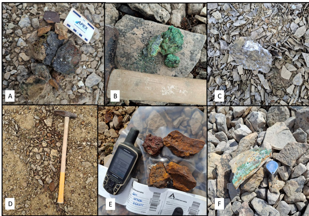
Figure 6: Examples of the interpreted copper gossans and outcrop from the Storm-Tornado area. For detailed descriptions of samples A-F above, see Table 4 in this report. Portable XRF was used to aid visual identification and these samples have not yet been analysed by laboratory.
