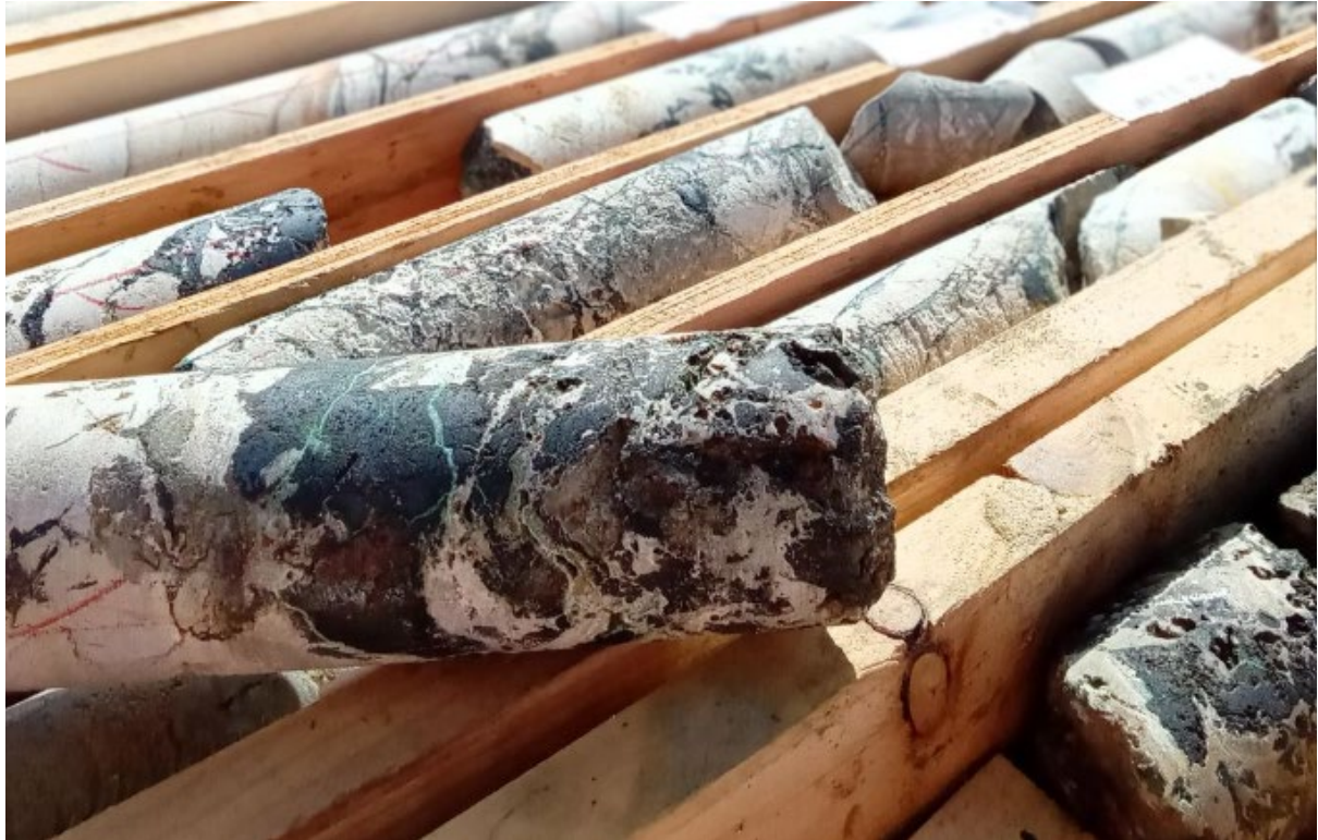
Figure 1: Diamond drill core from drill hole PFS-002. The core is from approximately 74m downhole and contains semi-massive visual chalcocite (dark grey mineral) within dolomite host rock (light grey). This interval has not yet been sampled and assays are expected in the next 6-8 weeks.
