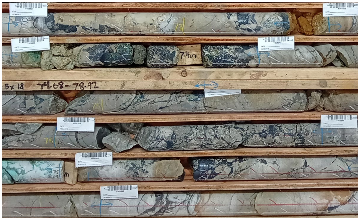
Figure 4: Dense semi-massive and breccia visual chalcocite (dark grey mineral) from PFS-002 (72.7-78.6m downhole). Assays for this interval are pending.
