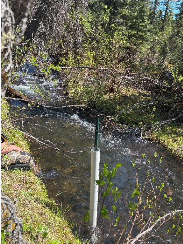
Picture 1. Greenbrush brook: staff water gauge installation
