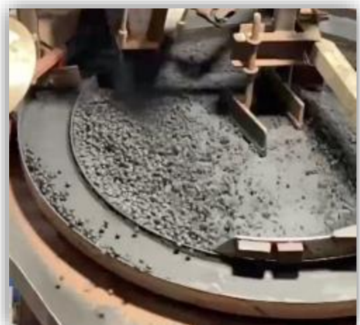
Picture 2. Green Ball manufacture in pelletising disc
