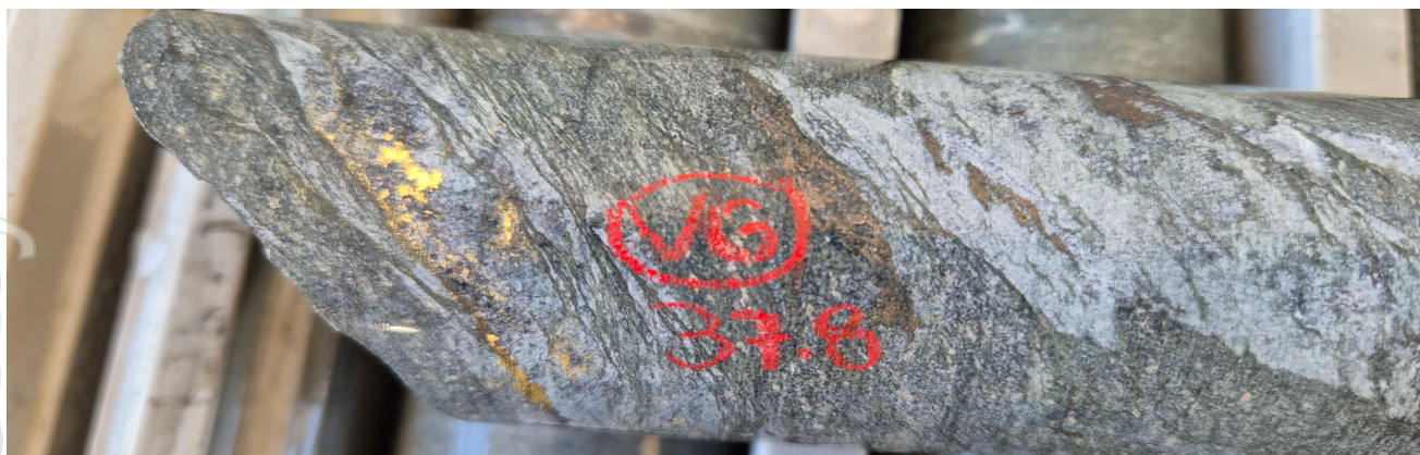
Figure 2: Core photo of visible gold from drillhole 25PGGC087 (37.8m). Trace amounts (<0.1%) of visible gold was logged within a small shear zone in the Gabbro. The shear zone was logged at being ~1m wide and the visible gold was located near the middle of the shear zone. The shear zone also contained ~5% disseminated, sheared pyrrhotite. Assays are pending for this interval and are expected in August 2025. Note: visual estimates of mineral abundance should never be considered a proxy or substitute for laboratory analyses where concentrations or grades are the factor of principal economic interest. Visual estimates also potentially provide no information regarding impurities or deleterious physical properties relevant to valuations. 13
