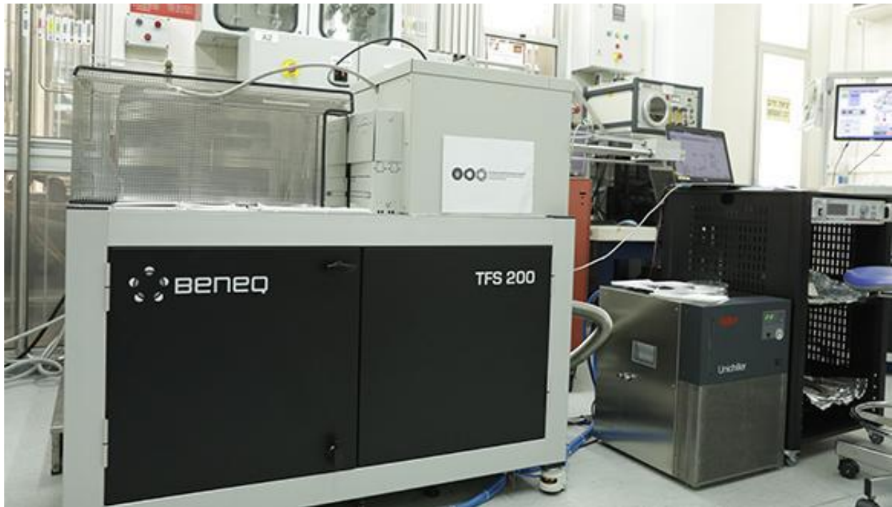
Figure 2: the Beneq TFS 200 ALD system at the Tel Aviv University's Jan Koum Center for Nanoscience and Nanotechnology
