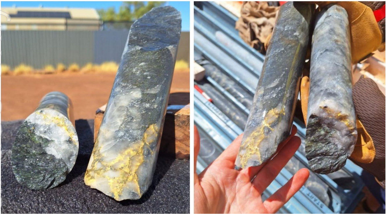
Figure 3: Visible Gold in Quartz - Carbonate Vein (intersected at 252m down hole in NGGRCD974 within a broader 16m wide shear zone)
