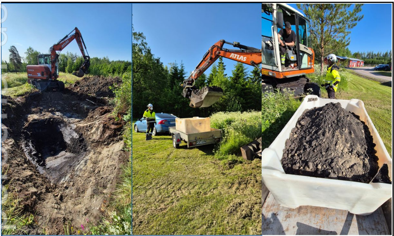
LnCS bulk sample collection in progress. Image does not purport to represent grade or mineral distribution.
