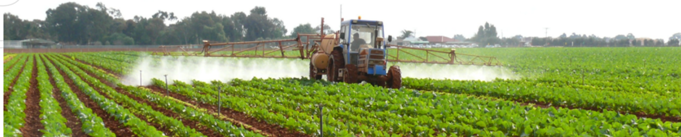
Figure 2: A boom sprayer applying liquid products to a lettuce field in Gingin, WA.
