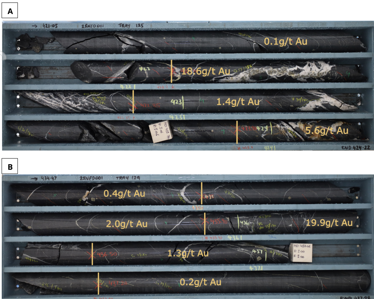
Figure 1 – Examples of high-grade drill intercept from Comstock Prospect DD hole 25NED001 (refer Table 1 on page 3 for full details of assay results). A) Tray 125 B) Tray 129.
