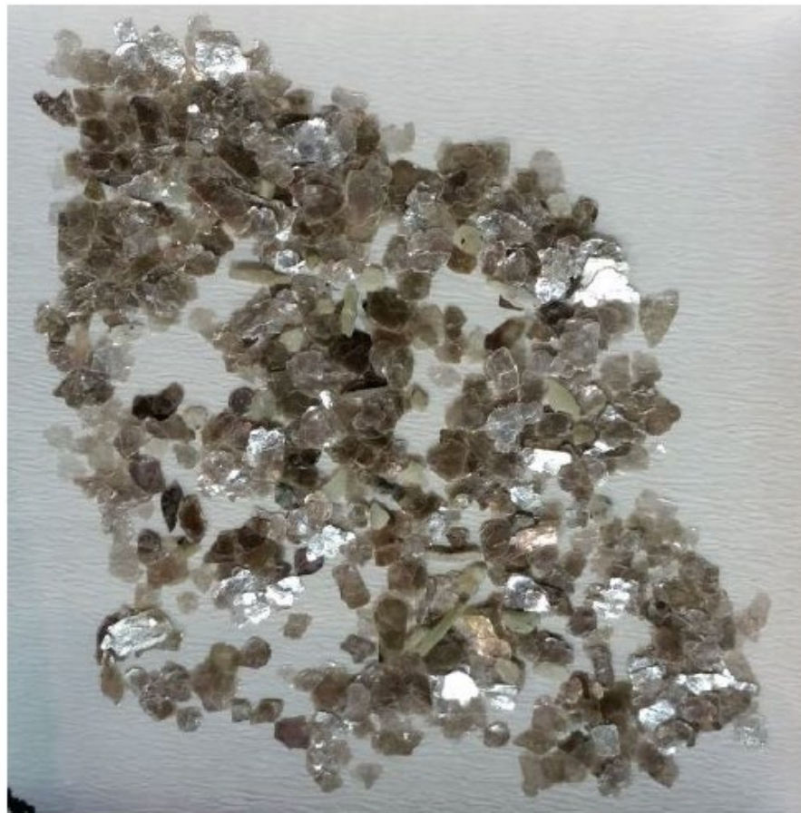
Figure 1: -3.35mm Stage 2 DMS Sinks Mica Laser Ablation Results from DMS test work report undertaken by Independent Metallurgical Operations Pty Ltd (IMO)
