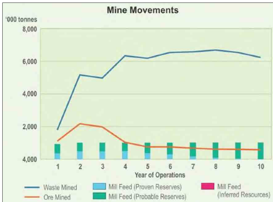
Figure 2-16: Mine Material Movement Schedule (Based on 2018 DFS)
