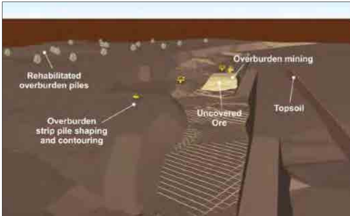
Figure 2-15: Illustration of Strip-Mining Progression (Optima, 2018)
