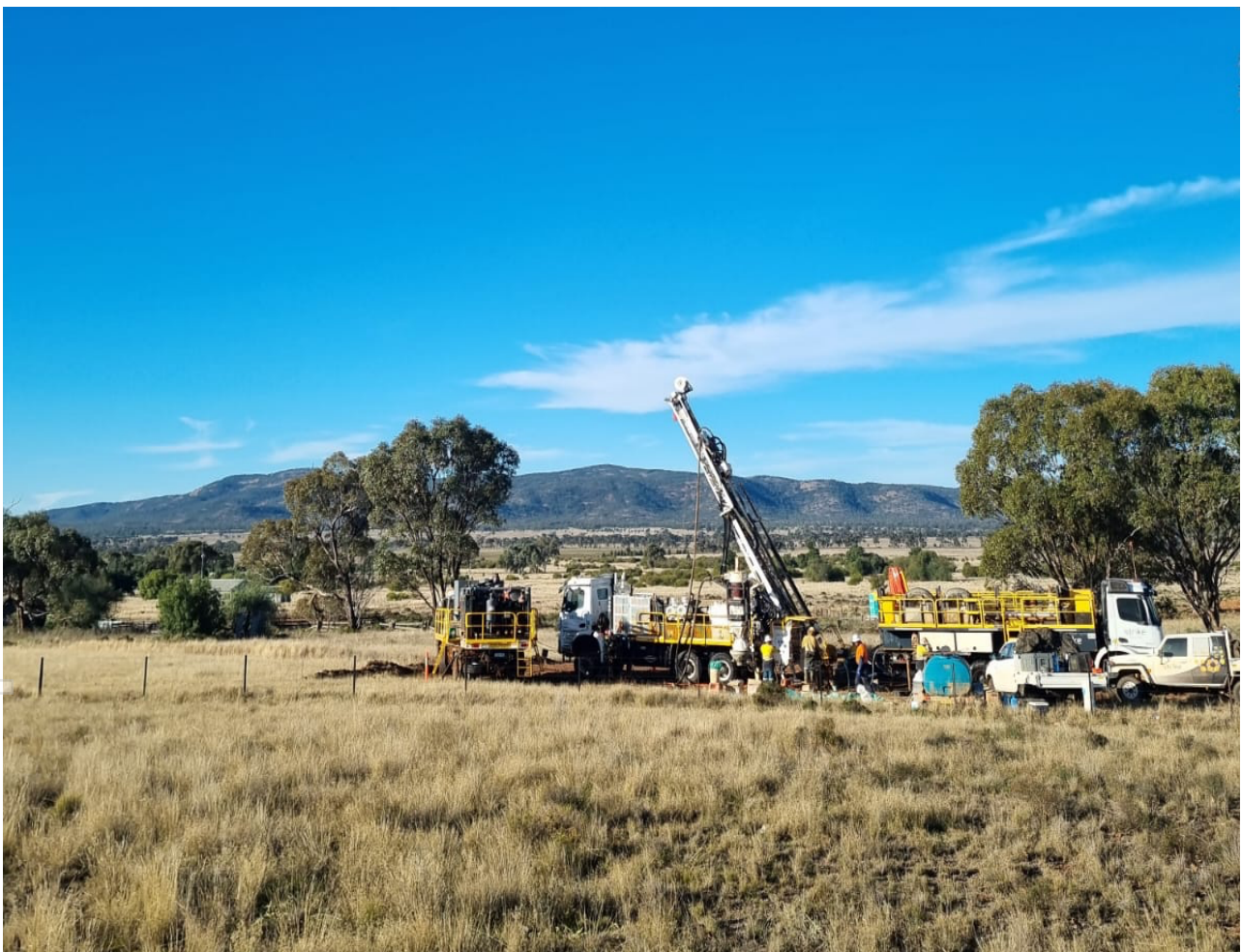
Figure 1. Strike Drilling RC rig drilling at Sheeppark Prospect
