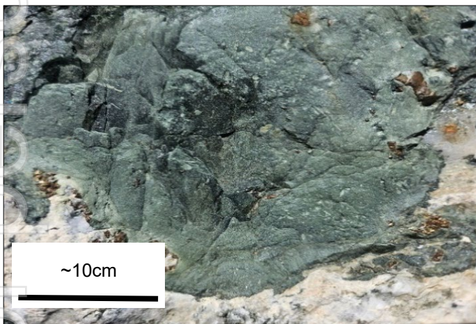
Image 3* (left) – Green schist foliation-hosted chalcopyrite and coarse pyrite within quartz veining. Image 4* (right) – Foliated black schist with groundmass hosted chalcopyrite and pyrite inclusions.
