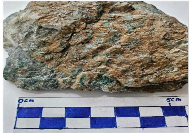
Image 1* (left) – Phyllite with quartz veins and malachite. Subhedral oxidized pyrite also present. Image 2* (right) – Weathered phyllite with malachite overprint and oxidized pyrite inclusion.
