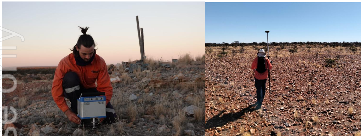
Figure 5: Photographs of Atlas Geophysics conducting non-ground disturbing ground gravity surveys at Ives Find Ongoing Exploration at Yandal West
