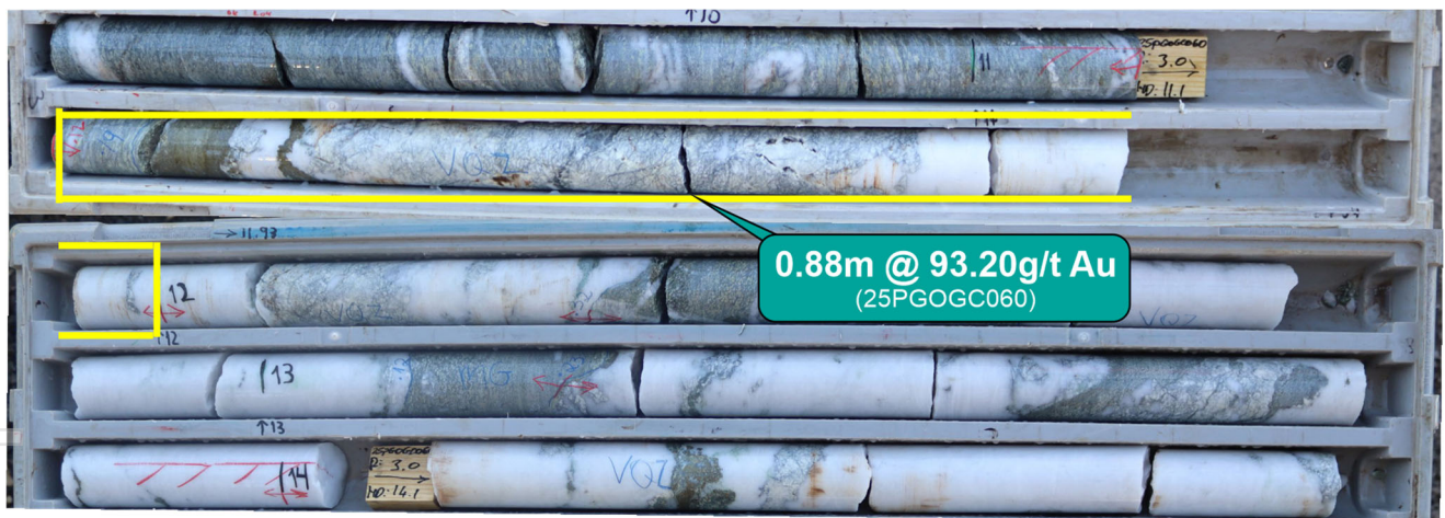
Figure 1: Core photo of 25PGOGC060 showing the intercept of 0.88m @ 93.20g/t Au (from 11.12m) within the Main Zone.
