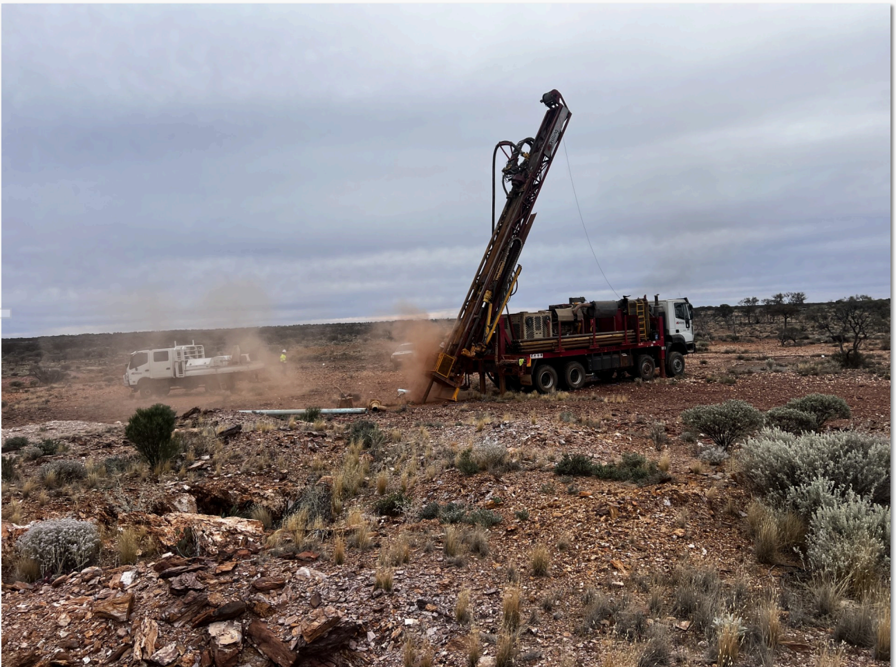
Picture 1: Drill rig at Sunday aligned to test beneath historical workings.
