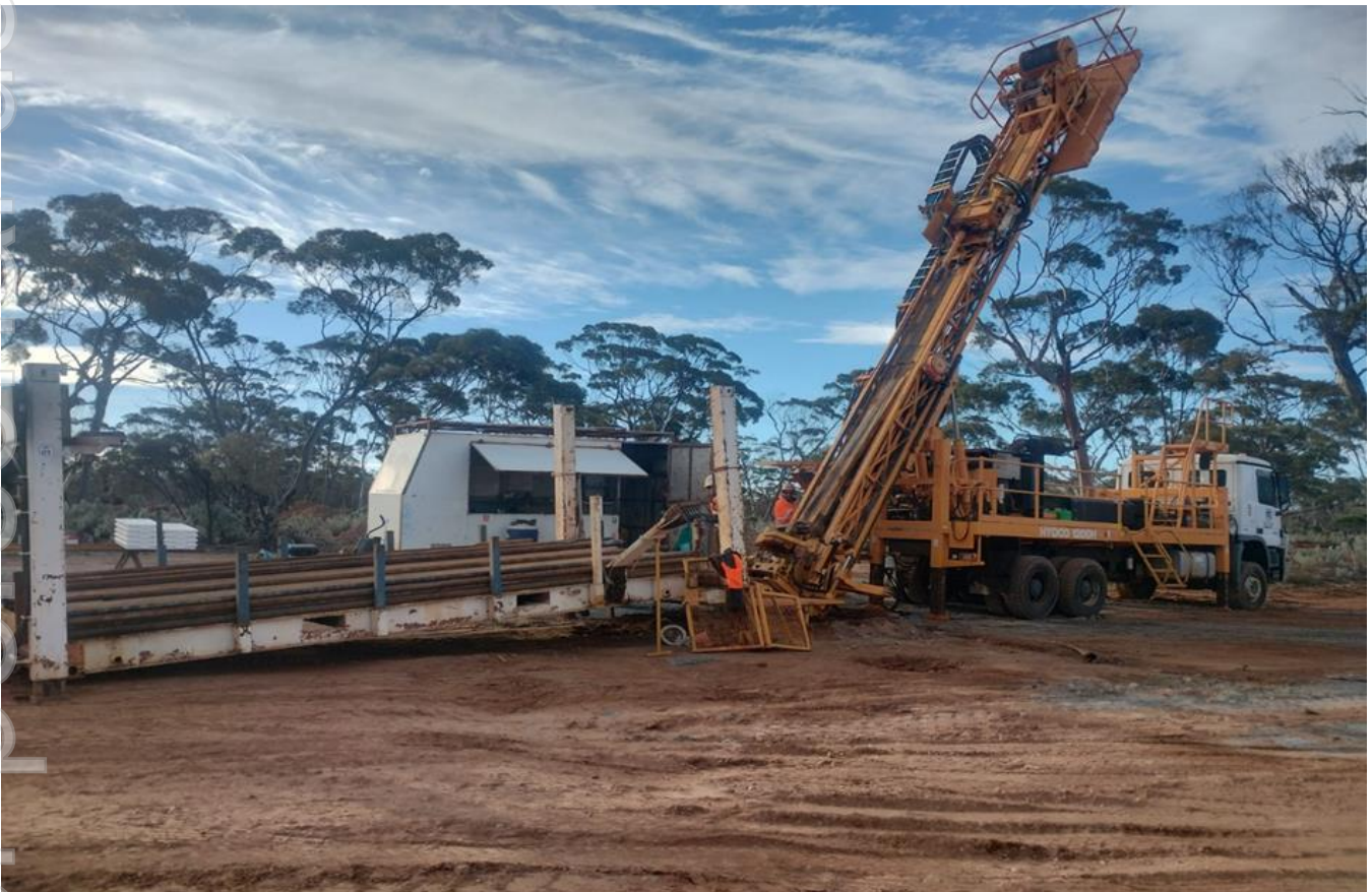
Figure 2 Diamond drilling is underway in hole 25PRC206 at the Paris Gold Project.
