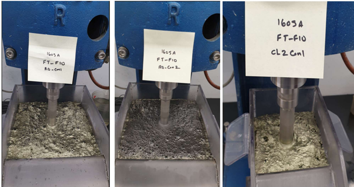
Figure 7: Copper concentrate from fresh composite, with chalcopyrite as the major copper mineral
