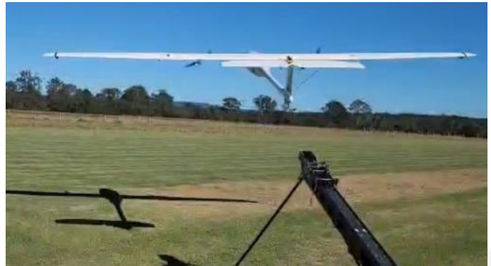
Pegasus I being tested from the catapult launch system
